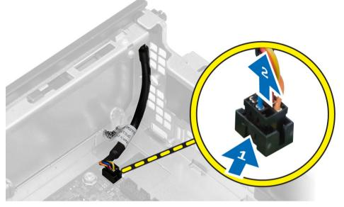
**4.** Press the clips on both side of the power switch to release it from the chassis and remove the power switch along with its cable from the computer.
