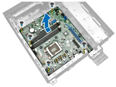
6. Tilt the system board at 45–degrees, and then lift the system board out of the computer.
