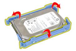
5. Remove the screws that secure the mini hard drive to the hard-drive bracket and remove the hard drive from its bracket.
