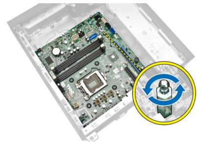
5. Remove the screws that secure the system board to the computer and slide the system board towards the front of the computer.
