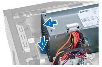
7. Lift the power supply out of the computer
