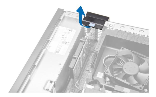
**4.** Pull the release lever away from the expansion card until you release the securing tab from the dent in the card. Then, ease the card up and out of its connector and remove it from the computer.
