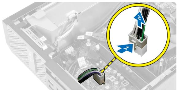
4. Disconnect the 4-pin power cables from the system board.
